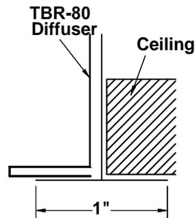
The PF-TBD slot diffuser mounting frame can be used in sheetrock or plaster ceiling. The frame is mounted in the ceiling by others. The Model TBR-80 is mounted on the inside lip of the frame. Plaster frame is 1 1/2" high.
